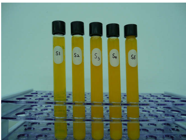
Fig. 1. Spherical- \text{Cu}_2\text{O} nanofluids 24 h after their preparation ( \text{CuSO}_4 molar concentration from 0.01 mol/L to 0.05 mol/L).
